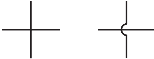
Figure 4-8: Nonconnecting crossed wires
