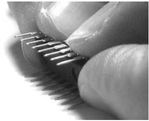
Figure 11-12: Bending the microcontroller pins
