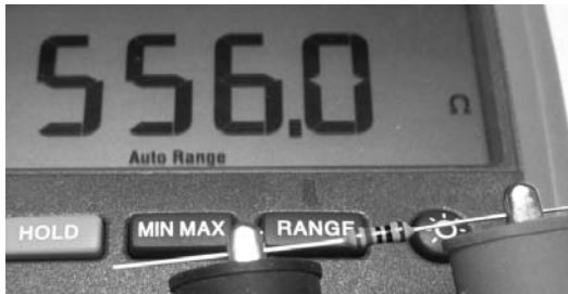
Figure 3-4: Multimeter measuring a 560-ohm 1 percent tolerance resistor
