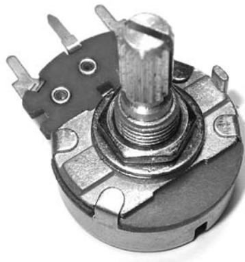
Figure 4-35: A typical linear variable resistor
